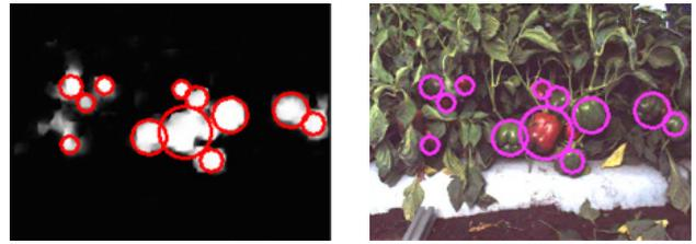
Fig. 4. Left is the probability map  $M(x, y, \sigma)$  indicating which pixels, for the image on the right, is most likely to be a sweet pepper. Circles in both images are the detected sweet peppers using the LoG region detector.
