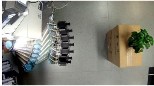
Fig. 8. An overview of the testing environment. The camera on the arm is moved across a set trajectory to capture images of the sweet pepper with varying levels of occlusion.
